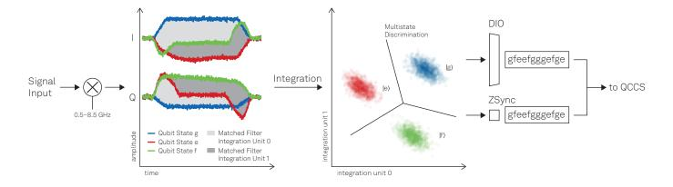
SHFQA analysis chain for a qutrit readout. After analog and digital down-conversion, the matched filters are used to achieve the maximum separation of qubit states g, e and f, then it will be discriminated and the digital bits are ready for feedback experiments.
